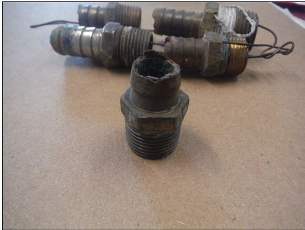
Fig. 6 Corroded Hose Fitting
