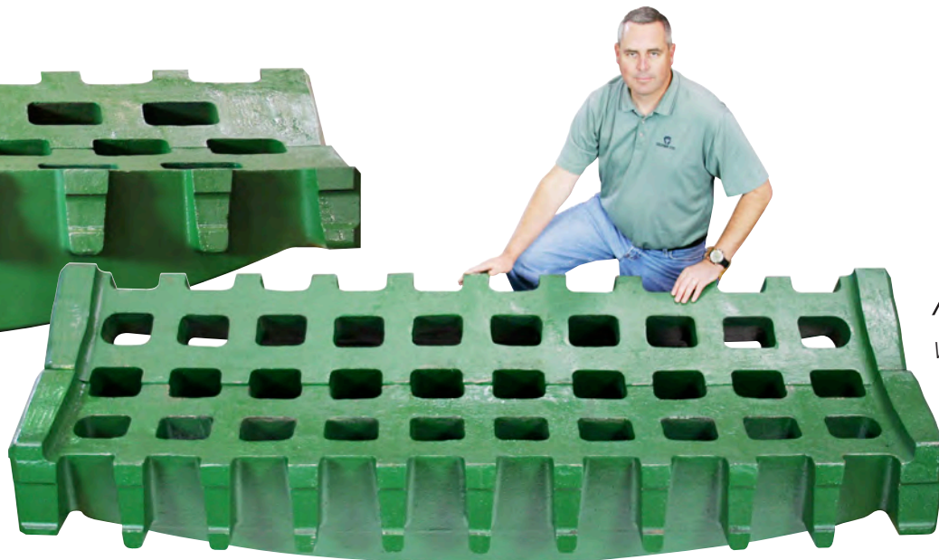
TSI 80 & 98 x 104 with staggered openings
